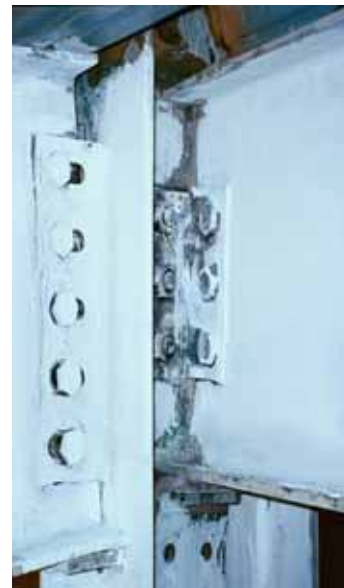
Figure 5.11. Yielding and Deformations without Fracture in the Connections, Test NSF-1 Progressive Collapse Prevention of Steel Frames with Shear Connections
