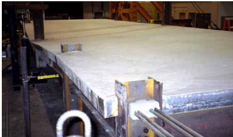
Figure 4.7. Displacement of Drop Column, Test GSA-1
