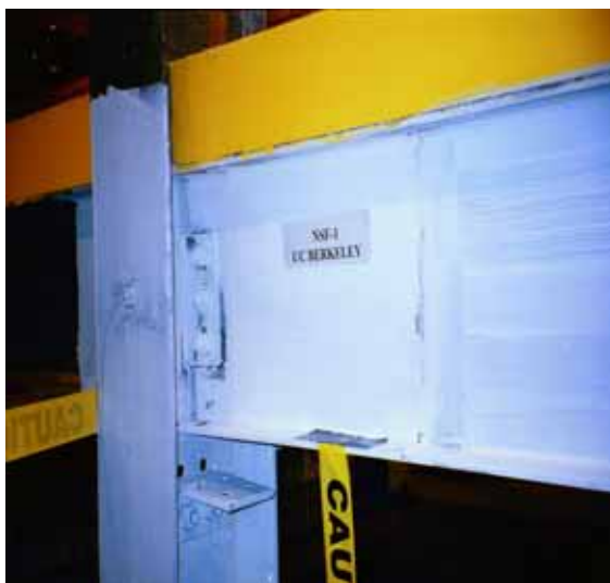
Figure 5.11. Yielding and Deformations without Fracture in the Connections, Test NSF-1 Progressive Collapse Prevention of Steel Frames with Shear Connections
